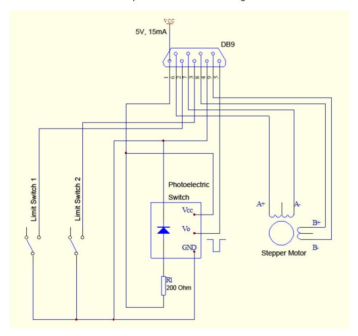
Limit Switch 1 is at the opposite end of the stepper motor. It's the home (zero) position.
